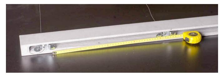
1. Measure precisely the distance between mounting holes (6 for 197cm, 4 for 162cm and 106cm) and mark them on the ceiling. Before measuring make sure mounting elements are positioned in one plane with the ceiling rose edges. If the ceiling surface requires it - install wall plugs.
